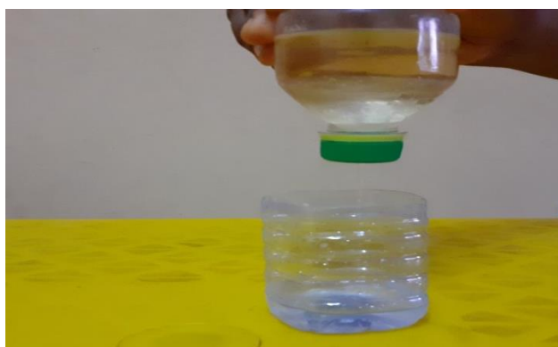
Fig 2. Water flows through the hole to separate it from the oil
